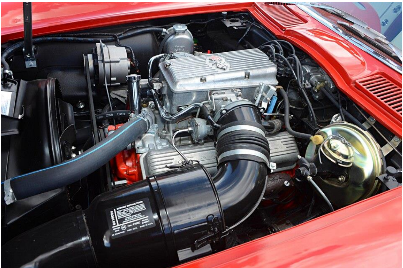
The fuel-injected 327 appears in its stock, 375-horsepower tune for racing.
