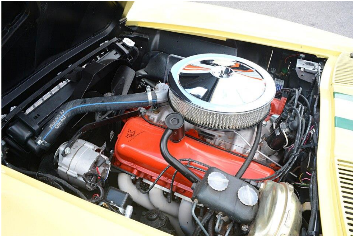
Alan Green pulled a 425-horse 427 (L72) off the lot to go racing. Joe Scafidi said, "Chevrolet sent them one of the HD 427 engines," which featured "12:1 compression ratio, heavy-duty rods, special camshaft and improved oiling."
