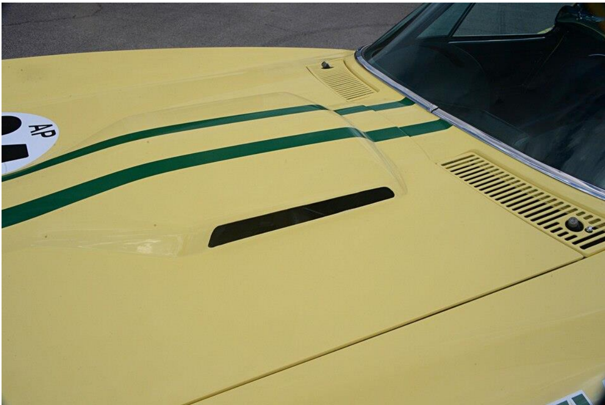
The bulge in the '66 hood is stock, but the sides are open for better airflow.
